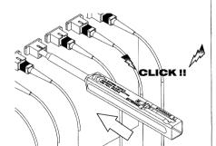
Be careful not to slant the Quick-Click SC Cleaner while inserting into the adapter.
