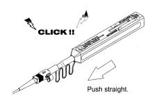
Be careful not to slant SC connector while inserting into the Guide cap.
