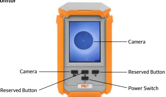
These monitors can be powered by an output 110-240V DC/AC or a rechargeable Li-ion battery equipped inside. Video input is dedicated to PAL/NTSC formatted probe. All of the display's controls are built into the handle for easy access.
