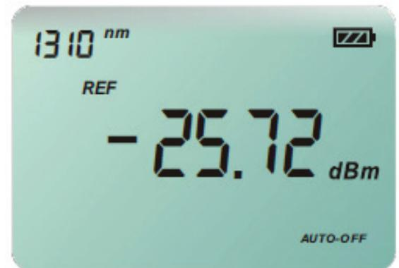
If the signal is greater than 1dB, push and hold the "UP" button to increase the current reference value in 1dB increments.
