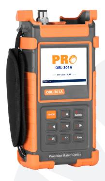
The OBL-301A is a high-performance, easy-to-use diagnostic tool designed for fiber maintenance, locating faults and general troubleshooting. The OBL-301A utilizes much of the same technology used in an OTDR, such as a graphical representation of the fault location, but at a much lower price point than an OTDR.
