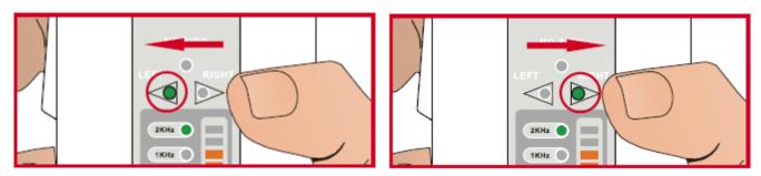
When no signal is present or the signal to be tested is too weak for the instrument to detect, the No Signal Indicator illuminates.
