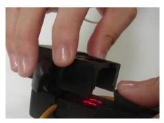
3) Slightly press the optical fiber into the slot of the shade cover and put it on the palm, then we can get the accurate measurement result.
