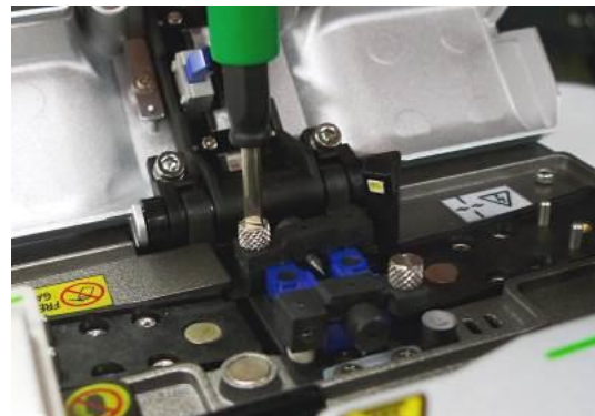
Fix electrode cover by tightening screws
