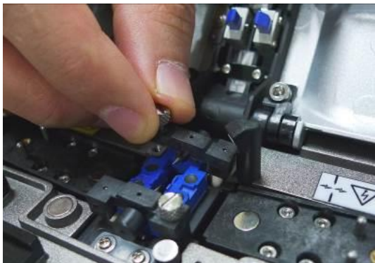
Correctly place an electrode into the V-groove of electrode base.
