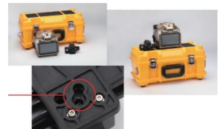
Fix cleaver to the worktable using screws
