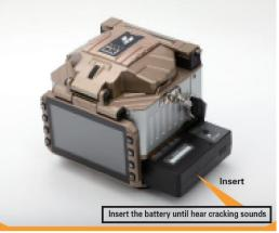
2) Use power pack which connects to the alternating current to do power supply, the method of install the power pack to fusion splicer is same as battery installation. Please refer to the following picture about power supply connection:
