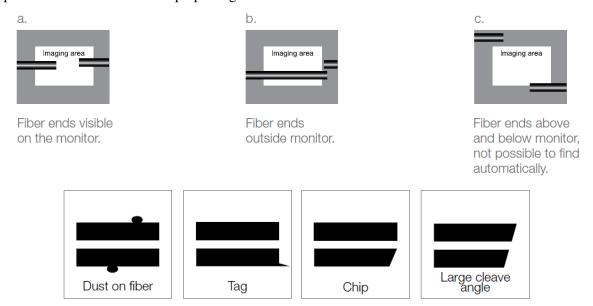
**Note:** The fibers are checked automatically when you press "Set" button. The splicer automatically focuses the fibers and checks for damage or dust particles.
