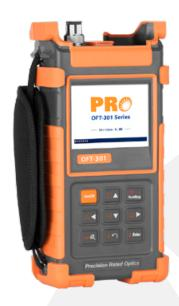
The OFT-301 Series OTDR is a high-performance, easy-to-use diagnostic tool designed for fiber maintenance, locating faults and general troubleshooting. The OFT-301 Series OTDR offers the same functionality as a high-end OTDR at a fraction of the cost.
