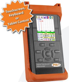
The OFT-3V Series OTDR can be controlled via Bluetooth from any Android device. Also included are a built-in Auto-Test /Auto-Wave Power Meter, VFL and CW/Fiber Identifier Light Source. An integrated Video Scope port is standard (scope optional).
