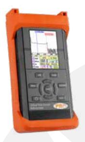
Manufactured in the USA, the OFT-CWDM-SB and OFT-CWDM-LB are ruggedized, compact OTDRs that are available in a variety of wavelengths, with up to four wavelengths per unit. The standard wavelengths are: 1471, 1491, 1511, 1531nm (SB) and 1551, 1571, 1591, 1611nm (LB). Other wavelength combinations are available upon request. The OFT-CWDM Series is water, dust and shock resistant, has onboard storage for 500 traces, video inspection capability and a USB port for easy data transfer.
