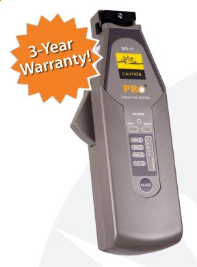
The OFI-11 Optical Fiber Identifier is a rugged, easy-to-use installation and maintenance instrument, which can detect low frequency tones at 270Hz, 1kHz and 2kHz. When traffic is present on the fiber under test, an audible tone can be heard. Fiber traffic direction is indicated by sequential LEDs on the probe.
