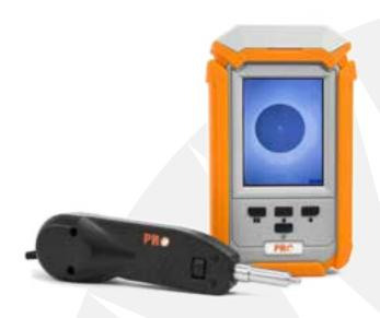
The VIP-35 Video Inspection Probe is designed to provide customers with the ability to troubleshoot network performance issues (most commonly caused by dirty connectors) by inspecting the end-face of a connector for debris. The VIP-35 includes a 400x inspection probe and a 3.5" TFT Active Matrix display for detection of even the smallest contaminants.
