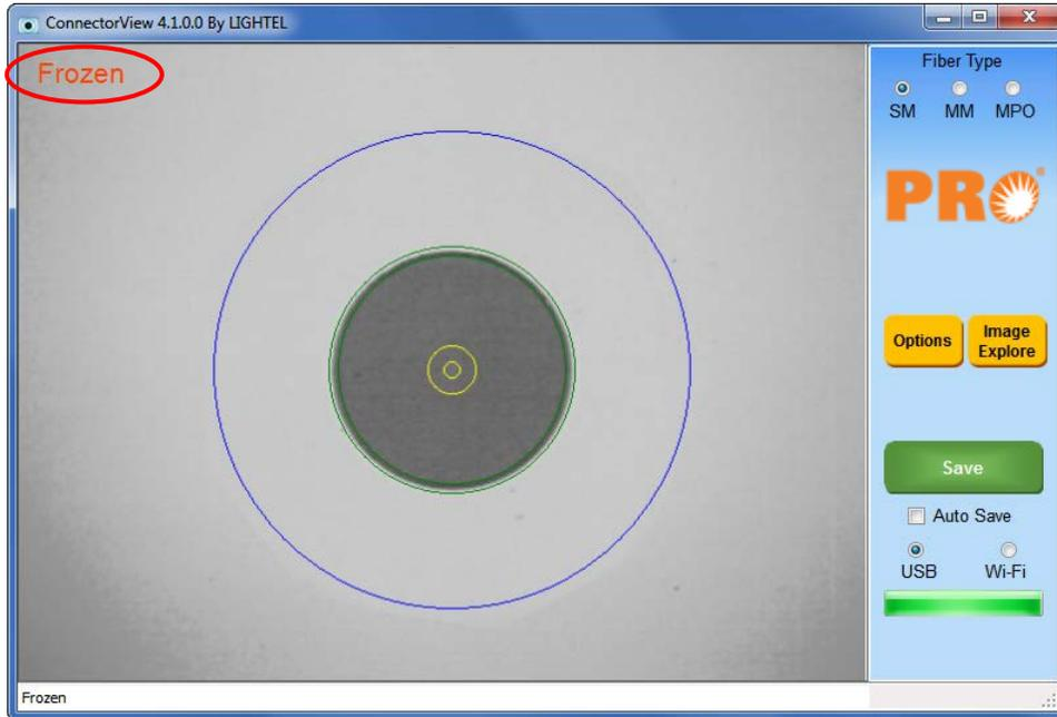
To save this frozen image click on the [Save] button or hit the [F10] function key on your keyboard. When an image is saved, the file name will be displayed in red in the upper left corner and the newly saved image will also be shown as the "Last saved image" along with its address at the bottom of the window.
