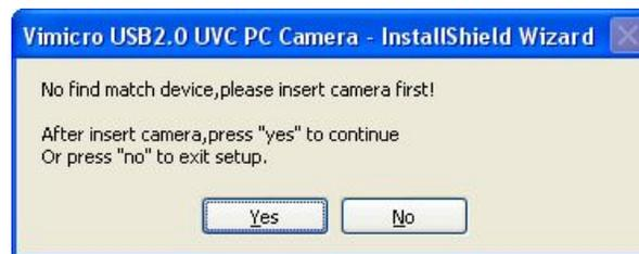
Plug the VIP-45 probe into one of the computer USB ports and click [Yes] to continue the installation.
