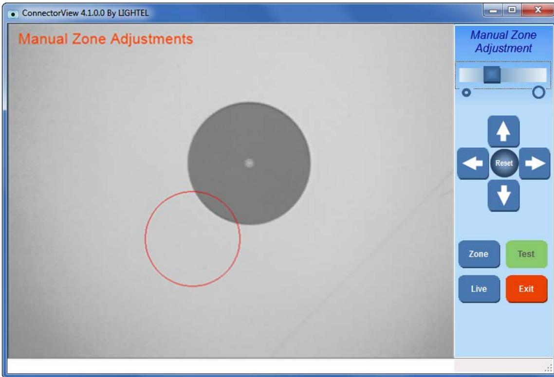
Use your mouse cursor to drag the red target circle to the right position. Use the slider to resize the circle, if necessary. Then use the arrows for fine position adjustments.
