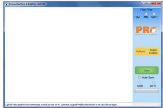
After properly connecting your device, click the “ConnectorView” icon to open the software. The USB or Wi-Fi radio button will be selected based on your type of connection.
