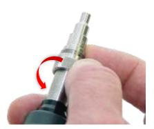
All tips have a slot and fit into the key at the top of the probe. Slide the new tip in place and slip the lock nut over
