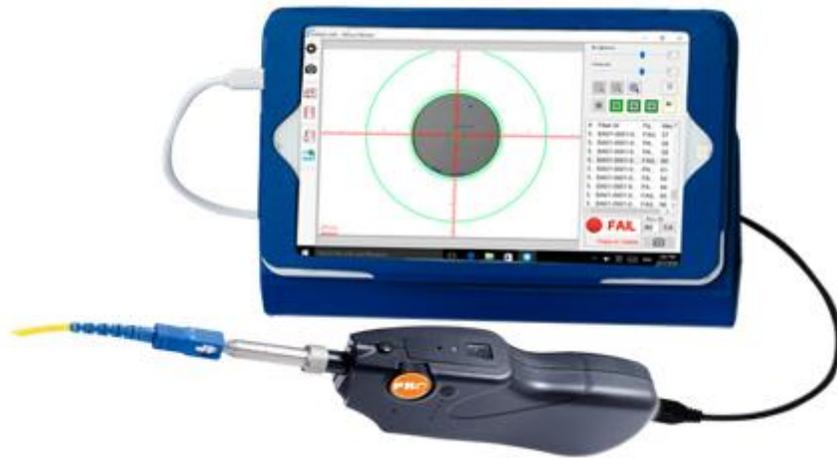
The fiber face analysis software FFA can be used to analyze the fiber end face image on Windows platform, it can have dirt, defects and scratches on the end face measured and recorded with pass/fail judgement. The latest version is 5.0, for more details, user can visit the company website for more information.
