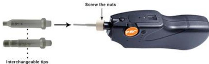
To mate different connectors, various tips are available and interchangeable. First loosen the retaining nut. Then remove the tips along the lens bar. Lastly make the change and tighten back the retaining nut.
