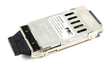
The WS-G5486 is programmed to be fully compatible and functional with all intended Cisco switching devices. This GBIC optical transceiver is based on the Gigabit Ethernet IEEE 802.3 standard. This module is designed for singlemode fiber and operates at a nominal wavelength of 1310nm.
