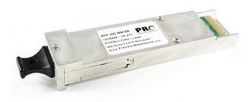
The XFP-10GER-192IRP is programmed to be fully compatible and functional with all intended CISCO switching devices. This XFP optical transceiver is designed for IEEE 802.3ae 10GBASEER, 10GBASE-EW, 10GFC and OC-192/STM-64 interconnects and is compliant with the XFP Multi-Source Agreement (MSA) Specification. This module is designed for single mode fiber and operates at a nominal wavelength of 1550nm up to 40KM.
