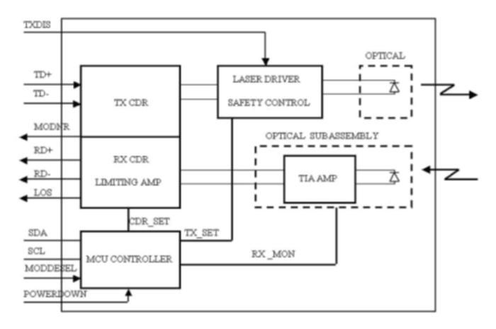
**Transmitter Section-** The Laser Driver accept differential input data and provide bias and modulation currents for driving a laser. An automatic power control (APC) feedback loop is incorporated to maintain a constant average optical power. Laser in an eye safe optical subassembly (OSA) mates to the fiber cable. TX CDR is used to overcomes host board and connector signal degradations by reshaping, regenerating, and attenuating jitter.
