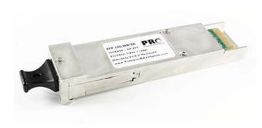
The XFP-10GZR-OC192 is programmed to be fully compatible and functional with all intended CISCO switching devices. This XFP optical transceiver is designed for IEEE 802.3ae 10GBASE-ZR, 10GBASE-ZW, 10GFC and OC-192/STM-64 interconnects and is designed to be compliant with the XFP Multi-Source Agreement (MSA) Specification. This module is designed for single mode fiber and operates at a nominal wavelength of 1550nm up to 80KM.
